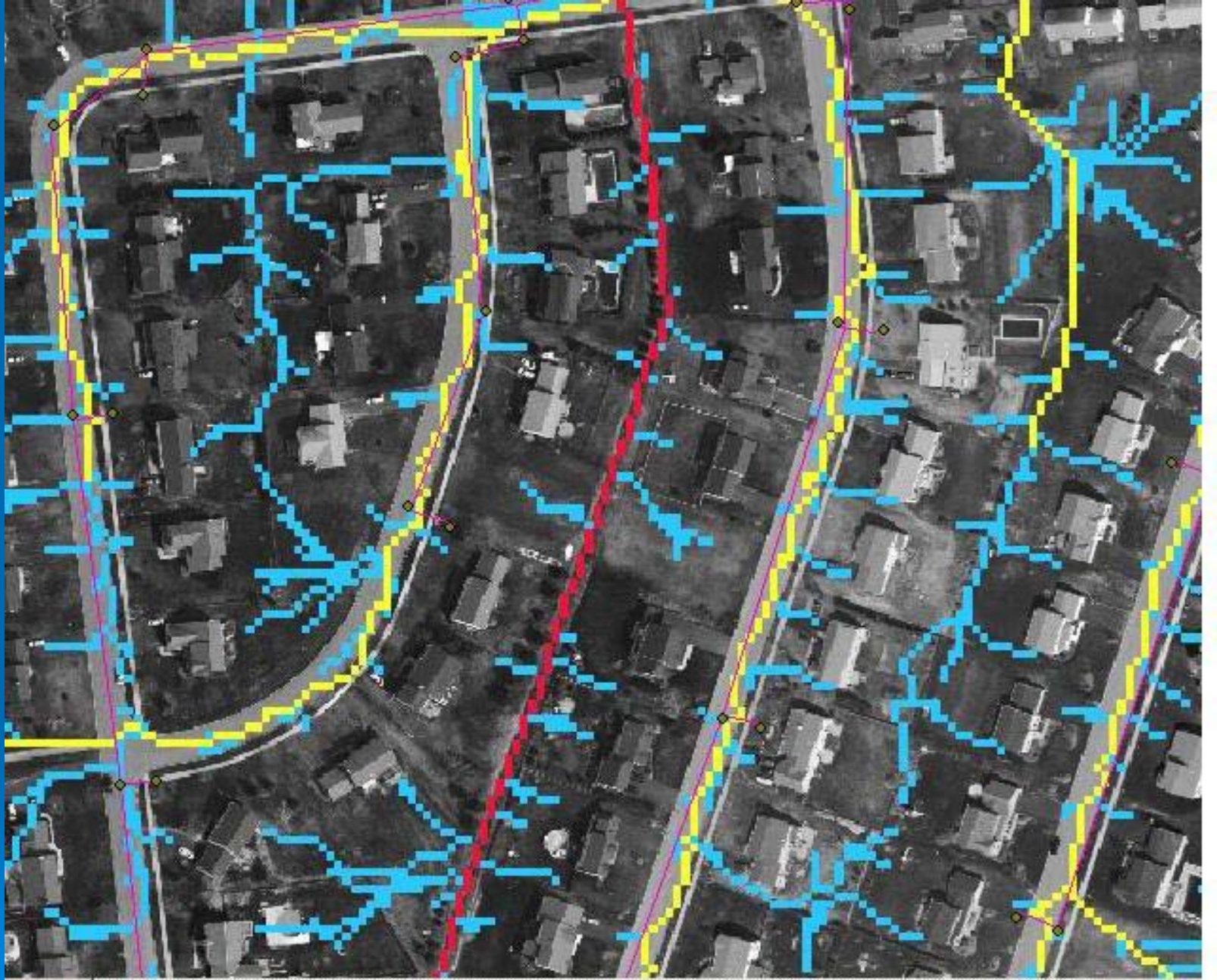
Closer look. Detailed storm micro-drainage
